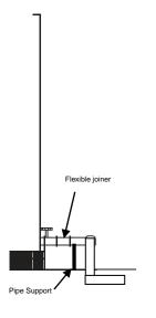
Unsupported pipework causes excess strain on fitting and tank wall.
