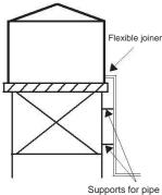
Placing tanks on stand. Use hardwood decking with gaps no greater than 10mm. Decking MUST be supported by bearers strong enough so as not to allow any deflection of decking when tank is full
